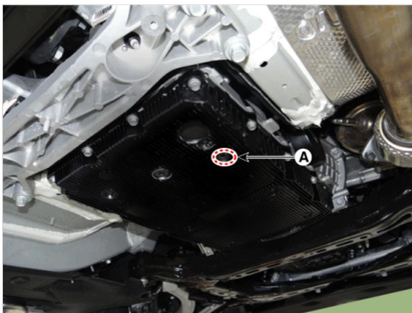
7. After ATF level check or exchange, be sure to remove ATF from outside automatic transmission.
